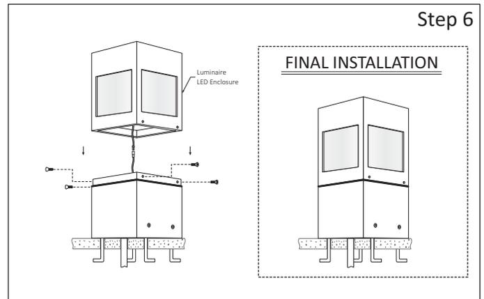
**Step 6 - Install Luminaire LED Enclosure:**
