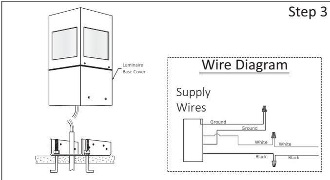
**Step 3 - Make Wiring Connections:**
