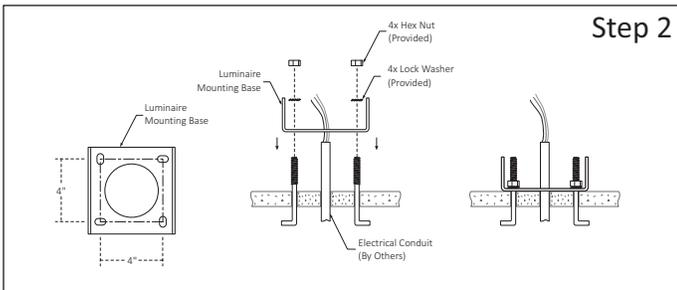
**Step 2 - Install Luminaire Mounting Base:**
